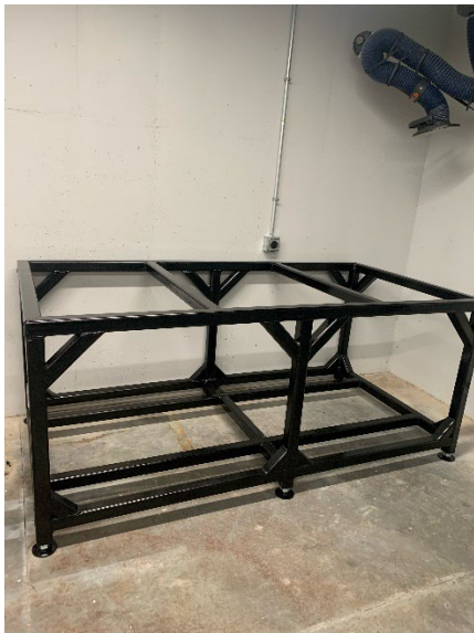
Figure 1: Steel support frame for road base test apparatus
